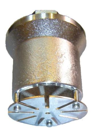
Each sprinkler is constructed with chrome plated bronze material and stainless steel deflector plate, which provides excellent corrosion resistance and can be easily used with sea water also.
